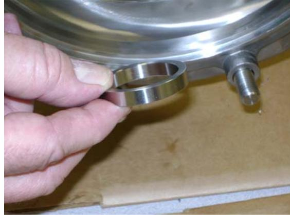
Align the pins on the rotating seal with the grooves on the seal driver and press the two components together. Wipe the seal face clean with a clean, soft cloth. Slide the gapping spacer onto the pump shaft. Note: it is important to use the same gapping spacer that was removed, as this is unique to your pump. This gapping spacer is what established the proper gap behind the impeller when the pump was assembled at Fristam.
