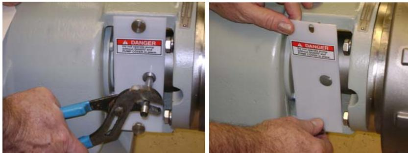
Remove the two water pipes from either side of the pump housing. Loosen the four guard screws and remove two plastic shaft guards from either side of the pump bearing block.
