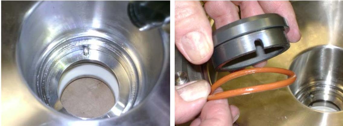
Turn the housing over and place it on the housing hub. Lubricate the stationary seal o-ring and place it on the new stationary seal. Place the stationary seal and o-ring into the bottom of the pump housing. Align the notch in the stationary seal with the pin in the housing. Press the stationary seal into the housing until it snaps into place. Wipe the seal face clean with a soft cloth to remove any oil or grit.
