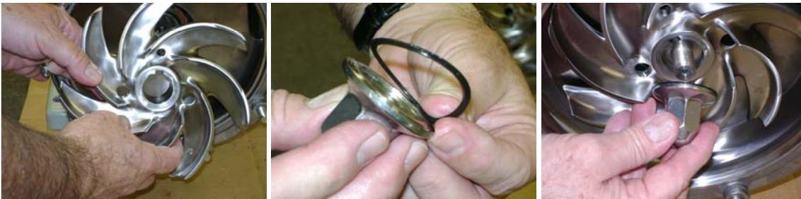
Slide the impeller onto the pump shaft. Lubricate the impeller gasket and place in the groove of the impeller nut. Thread the impeller nut with gasket onto the shaft.
