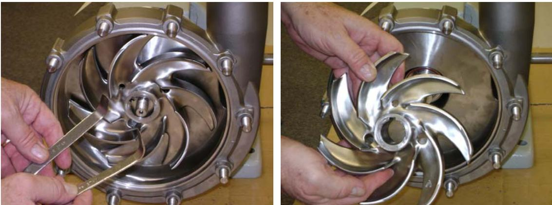
Remove the impeller from the pump shaft. Use impeller pullers to assist in removing the impeller, as needed. Be careful not to damage the threads on the end of the pump shaft.
