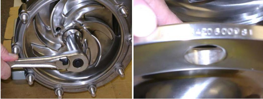
Place the chain wrench on the shaft near the coupling to keep the shaft from rotating while tightening the impeller nut with the 15/16" socket wrench. Tighten to 40 ft.-lbs. The picture at the right shows the pump serial number stamped on the side of the cover. Align this serial number with the matching serial number that is stamped on the pump housing when assembling the cover to the housing.
