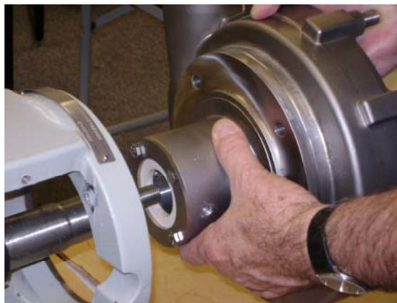
Carefully slide the pump housing over the pump shaft and push it against the bearing block, ensuring that the stationary seals (which are mounted in the pump housing) do not contact the shaft. Note: the stationary seals may be damaged if they make hard contact with the pump shaft.
