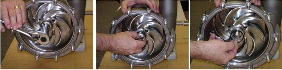
Place a chain wrench on the pump shaft near the coupling to keep the shaft from rotating while loosening the impeller nut with a 15/16" socket wrench. Remove the impeller nut and impeller gasket.
