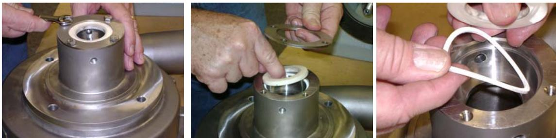
To remove the flush seal components, turn the housing over and place it on the housing studs. Remove the four retaining ring bolts on the housing with a 7/16" wrench. Remove the retaining ring, stationary water seal and flat gasket from the housing.
