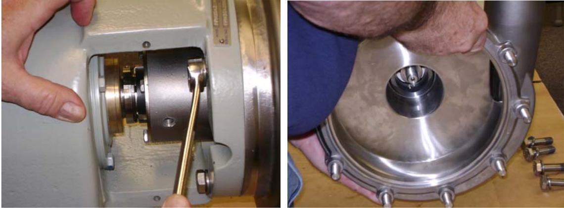
To remove the stationary seal and the flush seal components, the pump housing needs to be removed. Remove the four pump housing bolts and lock washers, which attaches the pump housing to the bearing block, using a 3/4" wrench. Carefully slide the pump housing off the end of the pump shaft, ensuring that the stationary seals (which are mounted in the pump housing) do not contact the pump shaft.
