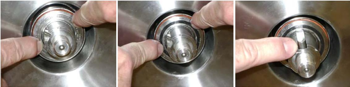
Lubricate the impeller gasket and place it into the groove on the seal driver. This gasket seals on the back side of the impeller. Place the impeller key into the shaft keyway.
