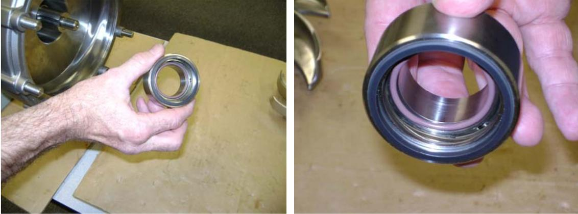
Slide the rotating seal assembly onto the shaft so the face of the rotating seal meets the face of the stationary seal.
