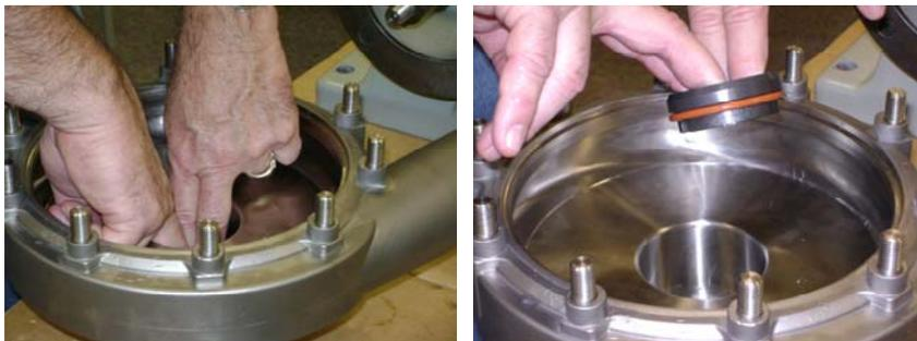
Place the pump housing on its hub. Remove the stationary seal by placing your fingers on the ID of the stationary seal and pulling it toward the front of the housing. The stationary seal o-ring should come out with the stationary seal.
