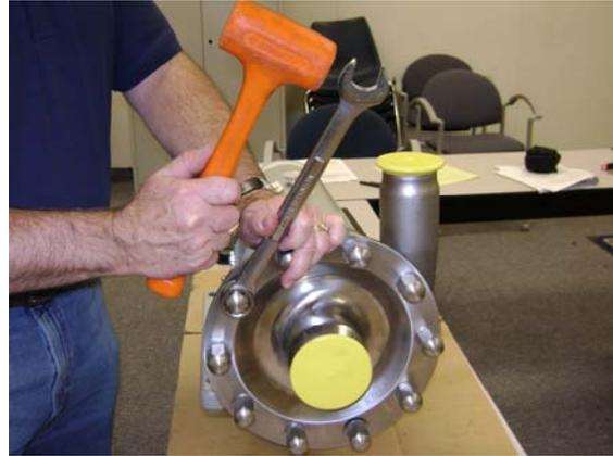
Install the cover onto the pump housing. Note: Align the serial numbers on the cover and housing. Place the flat washers and thread the cover nuts onto the housing studs. Tighten the cover nuts to 45 ft.-lbs. using a cross-tightening technique.
