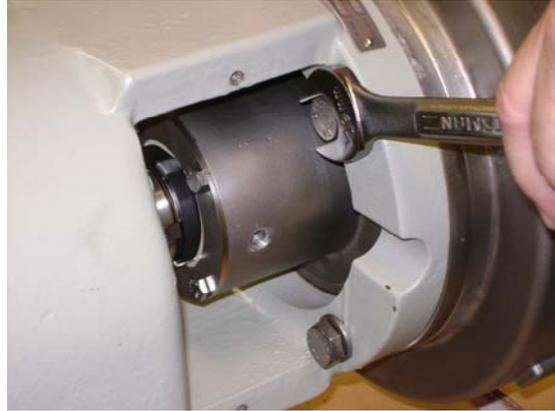
Check the rear water seal assembly and make sure the short tabs of the water seal drive ring are positioned in the slots of the water seal driver. Install the four pump housing bolts with lock washers through the bearing block into the pump housing. Tighten them with the 3/4" wrench to 55 ft.-lbs.
