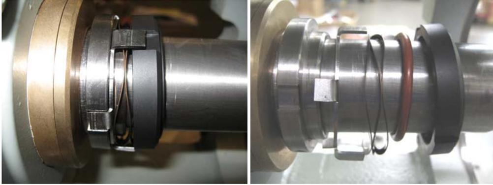
Now remove the rotating water flush components from the pump shaft, which include the rotating water seal ring, the water seal o-ring, the water seal spring and the water seal drive ring. The water seal driver may be left on the shaft.
