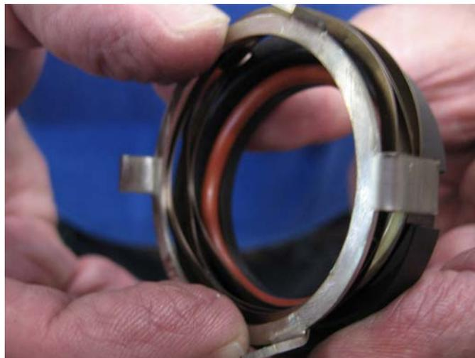
The above pictures show the components of the rotating water flush seal assembly. Note that the o-ring fits inside of the rotating seal ring. The longer tabs of the water seal drive ring fit into the slots on the outside of the rotating seal.
